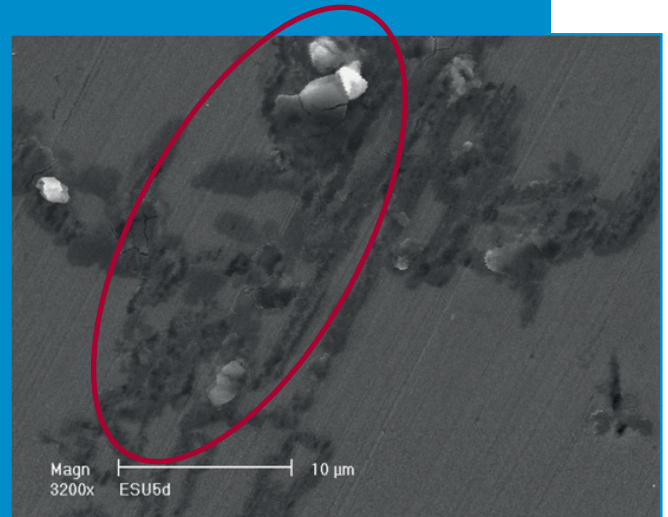
Figure 1, after (Wei Han, 2007): Scanning Electron Microscopy image of the surface of a steel plate exposed to atmospheric conditions for 5 days.(1)
